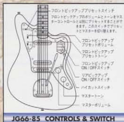
JG66-85 CONTROLS & SWITCH
