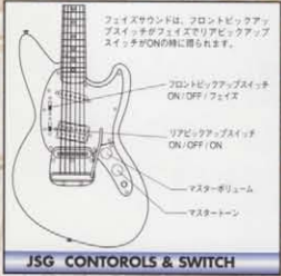
JSG CONTROLS & SWITCH
