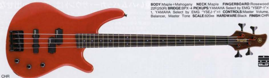
MB-55 ¥55,000 (税抜き) BODY:Basewood NECK:Maple(Scarf Joint/Bolt on) FINGERBOARD:Rosewood 22F(250R) BRIDGE:BPX-4B PICKUPS:YBS-F4PC(Ceramic)*1, YBS-F4JC(Ceramic)*1 CONTROLS:Master Volume, Master Tone, Balancer SCALE:820mm HARDWARE:Black FINISH:BL,WH,PRD,RBS
